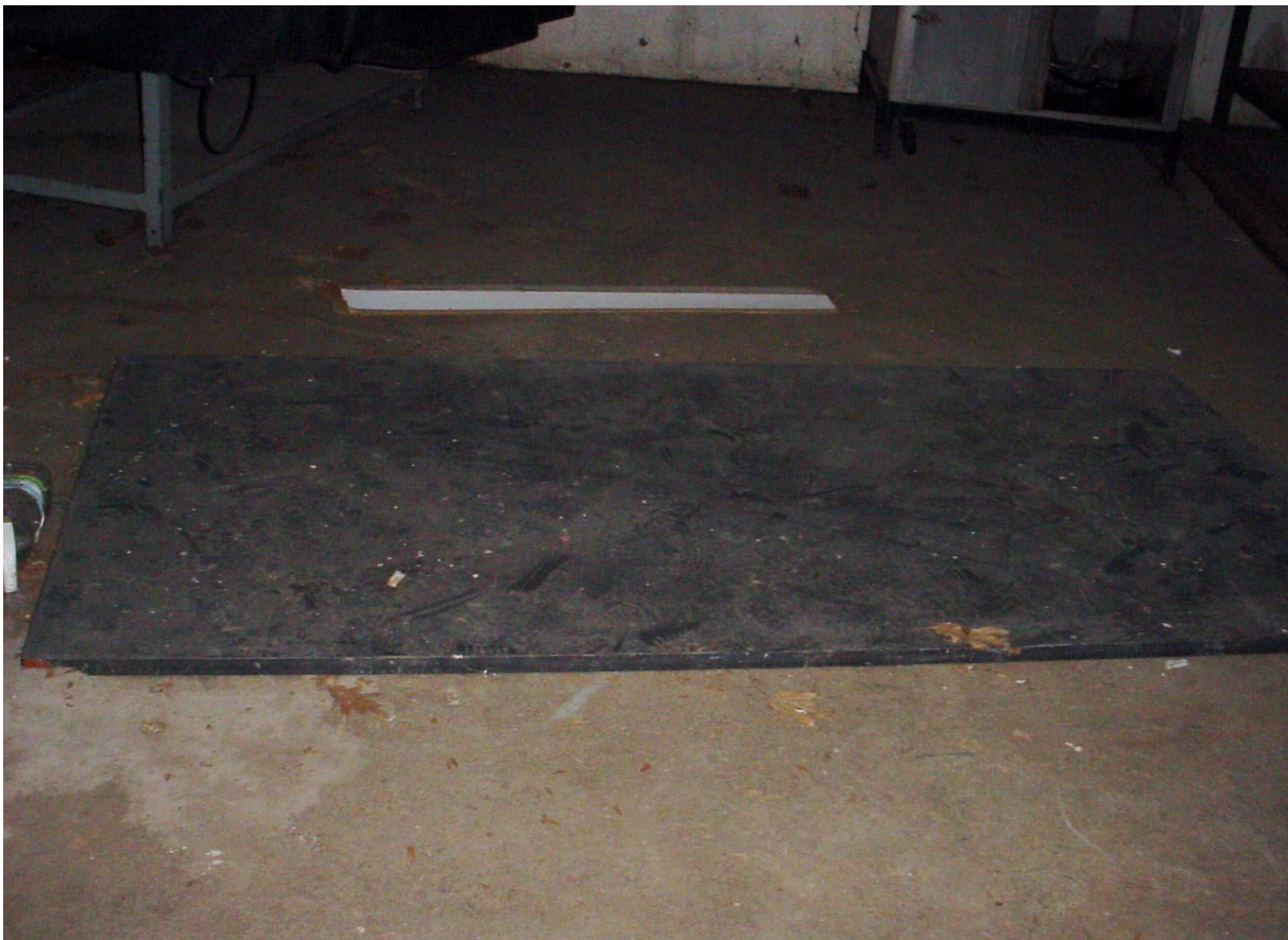
Photo #11: Asbestos-containing lab table top.
